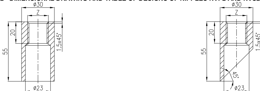
FIGURE 2 - DIMENSIONAL DRAWING AND TABLE OF DESIGNS OF NIPPLES NVP2 AND NVS2
