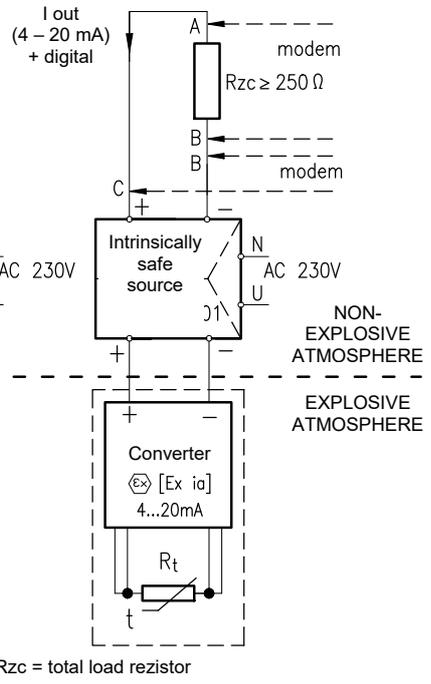
**FIGURE 3- EXAMPLE OF OPERATION CONNECTION OF TEMPERATURE SENSOR WITH CONVERTER IN LOOP 4 - 20 mA**
