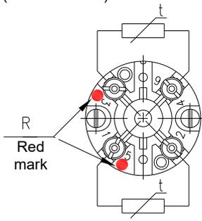
**D3** - With double measuring resistor in three-wire connection (2 × Pt 100/ I3)
