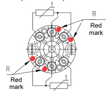
**SCHEME OF CONNECTION WITH CONVERTER AND DISPLAY**
