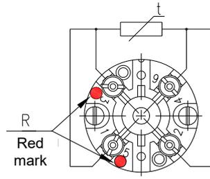
**D2** - With double measuring resistor in two-wire connection (2 × Pt 100/B/2)
