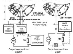
A–B and B–C are possible connection for HART modem or Communicator, max cable length Lmax see Table 2
