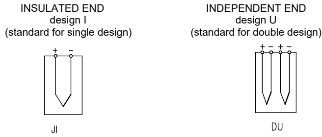
FIGURE 1 - DESIGN OF MEASURING ENDS OF JACKETED THERMOCOUPLES (SCHEMATIC ILLUSTRATION)
