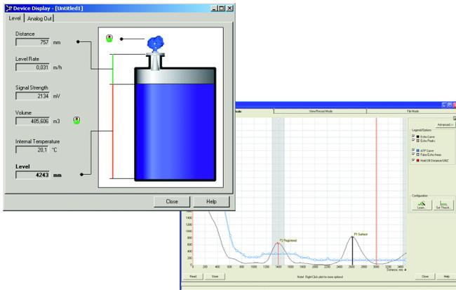
Rosemount Radar Master enables easy configuration and service with a wizard, an echo curve tool with the “Measure and Learn” function, offline/online configuration, an extensive online help, logging capabilities, and more.
