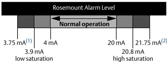
1. Transmitter failure, hardware or software alarm in Low position.
