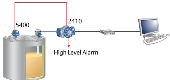
Independent alarm sensor in a continuous overflow prevention tank gauging system
