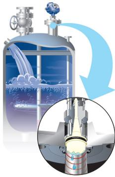
Larger sealing surface towards the process connection, making the transmitter less sensitive to condensation and dirt. Circular polarization will automatically reduce the disturbance effect close to tank walls and obstacles.
