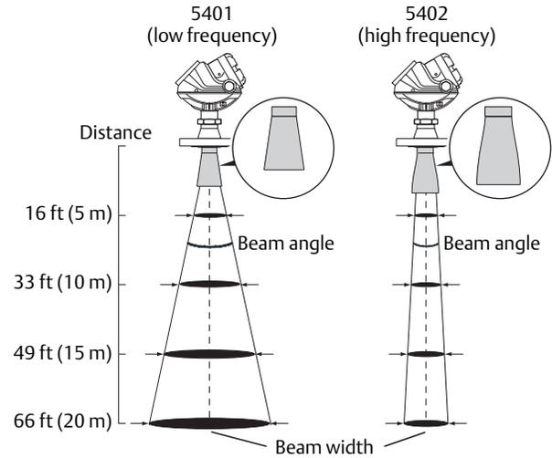
For a comparison between the beam angle and beam width for the Rosemount 5401 (~6 GHz) and 5402 (~26 GHz) transmitters with antennas of the same size and type, see the following tables.
