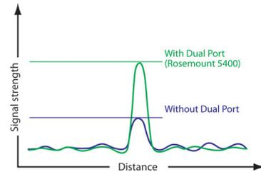
The unique dual microwave ports for sending and receiving radar signals yield a 75% stronger signal than single port transmitters.
