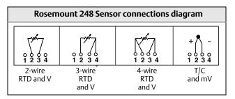
Rosemount Inc. provides 4-wire sensors for all single element RTDs. You can use these RTDs in 3-wire configurations by leaving the unneeded leads disconnected and insulated with electrical tape.
