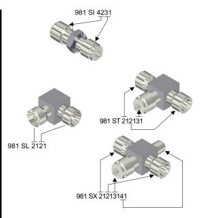
The coupling consists of the coupling body and terminals pursuant to Figure 18.
